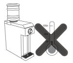
Do not install the unit in a place where there is direct sunlight or where the ambient temperature gets below freezing (32°F / 0°C) (risk of damage to the unit).
